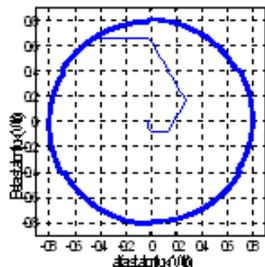
(f) Stator flux trajectory
