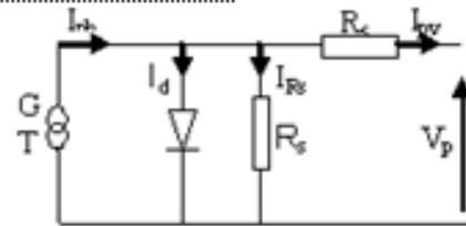
Fig.2. Simplified equivalent circuit of solar cell
