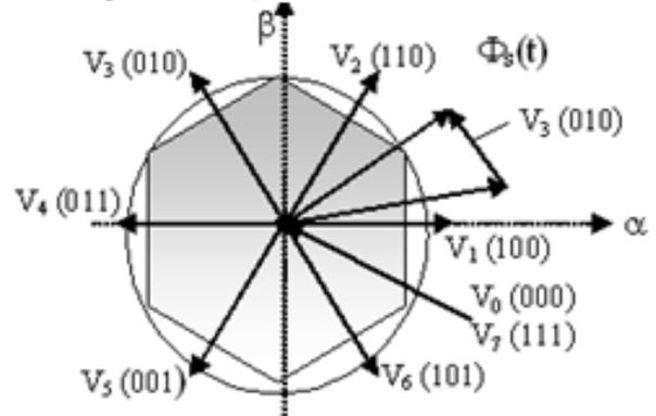
Fig.4. Movement of the inverter voltage in the space-vector plane
