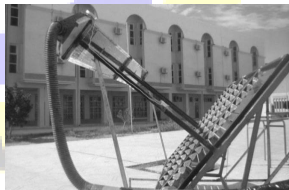
Fig.1: Linear Fresnel reflector solar concentrator with rectangular useful conduit absorber.
